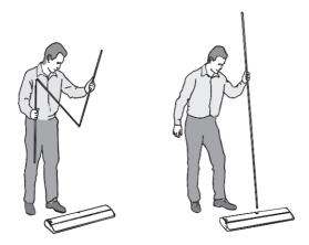
1. insert the assembled pole to the base hole
