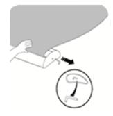
5. activate the spring tension by removing the Allen Key
