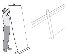
3. fix the hook of beam top bar to the 3-sectioned pole
