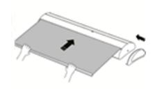
6. carefully allow the graphic recoll into the base unit, then reattach the cover
