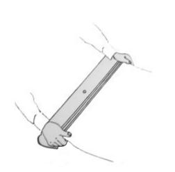
6. The inner spring is now armed, and will pull the banner into the base with great force. Carefully guide the print in with a hand on each side.
