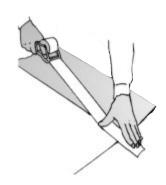
IMPORTANT: Reinforce the included Adhesive Strip by using a 2" packing tape, half on the print and half on the Leader.
