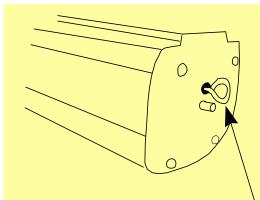
IMPORTANT - Do not remove the Locking Pin until the banner has been installed.
