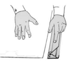
1. Open the clamping top bar by pulling the the flat front piece up and away from the back piece. This opens a slot along the bottom. down on the Top Bar to clamp.
