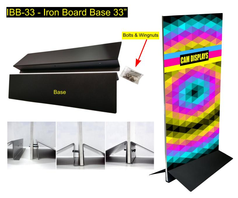
The IBB-33 has three 3/8" bolt holes that need to be pre-drilled in your rigid board before installation. Each hole is 1 3/4" from the bottom of the board. The center hole is 16 3/4" from the side, and the side holes are 4" from each side. The Board Base covers the bottom 3 1/8" of the board.
